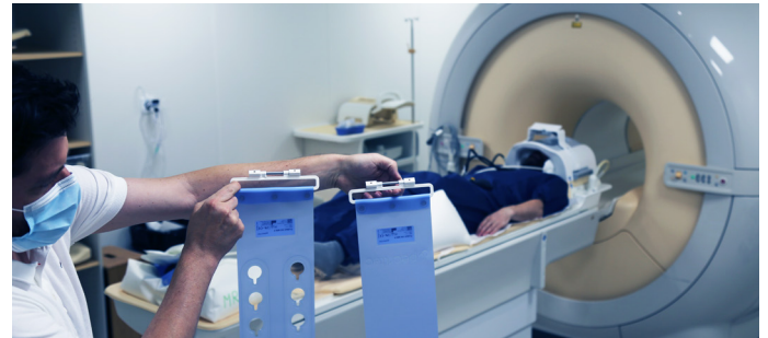
Figure 4: ProBelts are attached to the existing Philips mount (white eyelets) by means of snaps.
