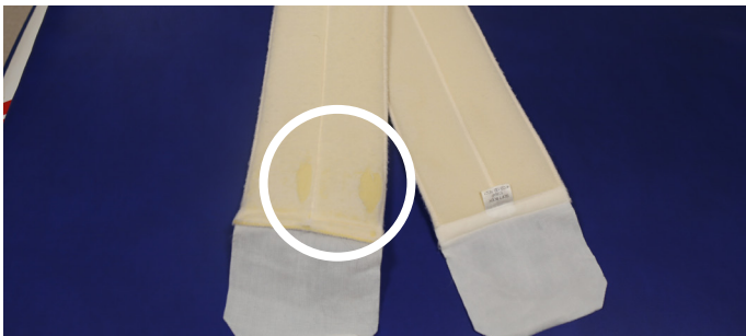
Figure 3: Due to continuous washing, the hook-and-loop system does not work optimally, and it makes the fixation belt look unhygienic.
